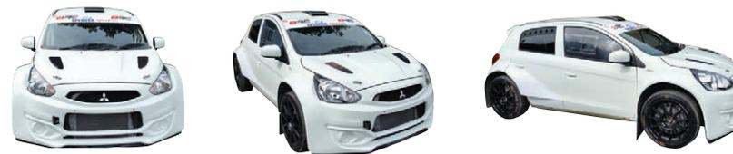
The Mitsubishi R5 is built precisely to FIA R5 Class specification. It features a 1620cc engine based on the Mitsubishi 4B11 unit from the Evolution X, connected to a five-speed Sadev transmission and four-wheel-drive system. The car is fitted with MacPherson suspension and Öhlins dampers all round, mated to specially designed subframes.
